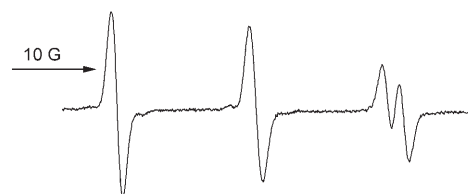
Figure 2. EPR spectrum of 4 (0.1 mM) recorded in the presence of CB7 (0.20 mM) at 298 K.
